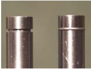
In Stahlhammer endpins, a missing rubber ring on the inner shaft can cause a buzz
