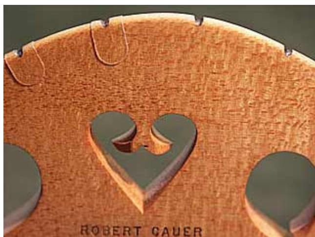
The notches are darkened with a soft pencil
