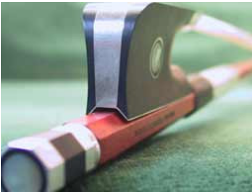
Loose eyelet resulting in frog warbling on stick
