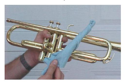
Valve casing brushes are made to clean valves. But here's something cheaper and easier. Go to a Chinese restaurant and steel a chopstick. Preferably a wooden one. These are absolutely perfect for the job since they have a rectangular surface on one end where you wrap a piece of cloth on it. Wrap the cloth around the thicker square end of the chopstick and then fold the cloth over the top.
