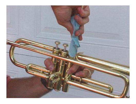
Do the same thing from the top. Insert the cloth form the top of the valve casing. After this your valve casing will be unbelievably clean.
